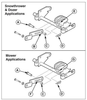
Figure 29. Lift Link - Manual Lift Models
